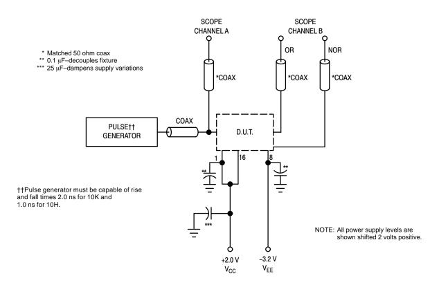
Figure 15. MECL Logic Switching Time Test Setup
