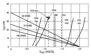
Figure 16. Output Voltage Levels vs. DC Loading (Load Lines for Termination to -2.0 Vdc 25°C)
