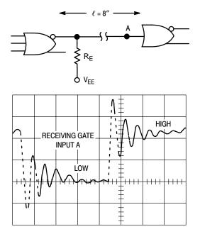
Figure 1. Unterminated Transmission Line (No Ground Plane Used)
