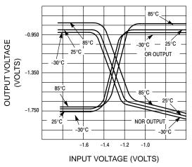
Figure 7. Typical Transfer Characteristics as a Function of Temperature (MECL 10K)
