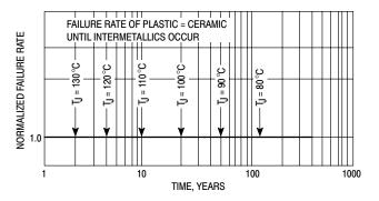
Figure 24. Failure Rate vs. Time Junction Temperature
