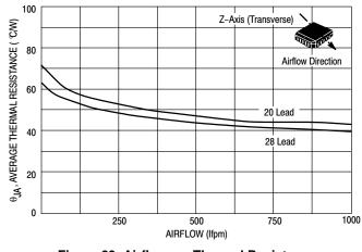
Figure 23. Airflow vs. Thermal Resistance (PLCC Package)
