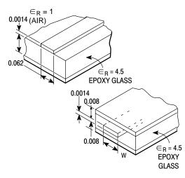
Figure 35. PC Interconnection Lines for use with MECL
