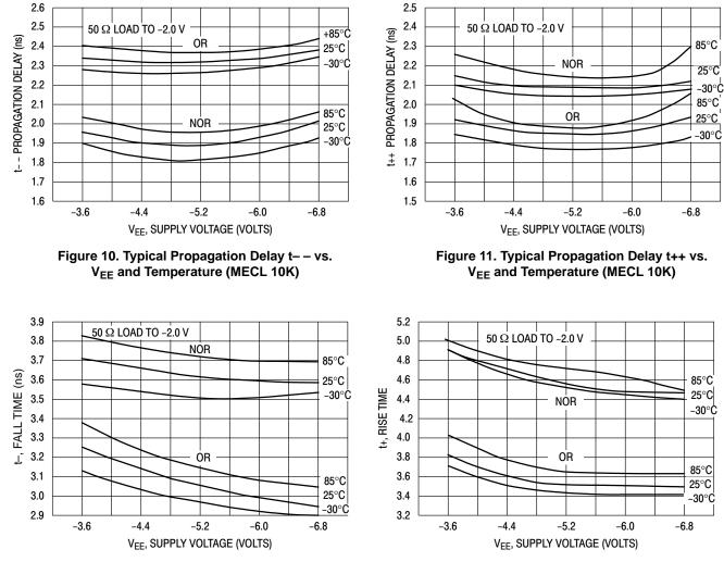
Figure 12. Typical Fall Time (90% to 10%) vs. Temperature and Supply Voltage (MECL 10K)
