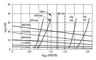
Figure 17. Output Voltage Levels vs. DC Loading (Load Lines for Termination to  $V_{EE}$  (-5.2 Vdc) 25°C)
