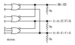
Figure 37. Use of Wire–OR and Complementary Outputs
