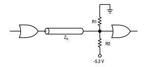
Figure 31. Parallel Termination – Thevenin Equivalent
